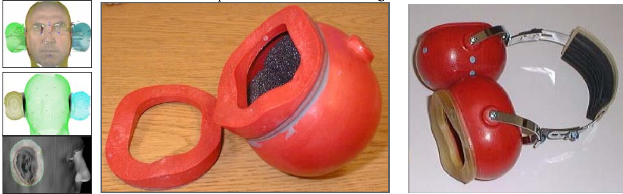
Figure 11 Head Shape Extraction and Resulting Custom Earmuff
